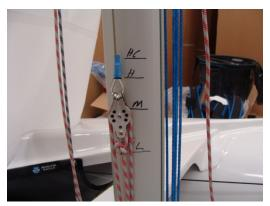
general rule of thumb should be to avoid luff sag as the breeze fills. Keep in mind that as you adjust your rake you must also adjust your bridle and vang to accommodate proper leach trim. The mast pin should be positioned in the second hole from the front.
