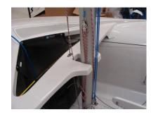
10. **Install jib sheets.** The jib sheets are black and clearly labeled in the line kit. First, fold the sheets in half to find the middle. Feed the middle through the grommet on the clew of the jib so that 3" come out the other side then put the two tales through the loop. Pull tight and lead to each side of the boat. The sheets will pass between the shrouds and trapeze. Feed them through the fairlead and be sure to tie a stopper knot.
