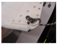
16. **Install the rudder & Tiller**. When you put the rudder on the pintles be certain that the rudder clip is engaged. This will prevent the rudder from
