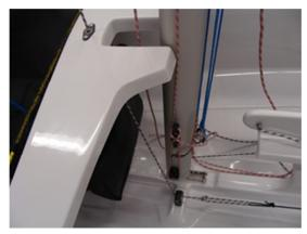
knot avoids being stuck in the fairlead. The hook should be adjusted with the spinnaker pole at maximum height and the knot that ties to the shock cord should bottom out at the fairlead. This will stop the pole from skying. Once the height of the hook is adjusted you might want to tie an overhand knot at the hook to secure the hook from slipping. The other end of the line will feed through the forward most cleat on the starboard side of the board cap.
