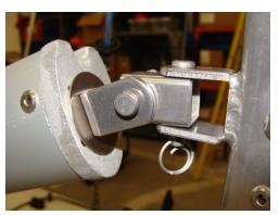
7. **Boom & Vang Connection.** Undo the pin at on the gooseneck and put it through the universal on the boom. Next attach the vang
