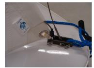
3. Attach the shrouds. The shroud adjusters are attached to the forged eye strap with the guy roller pin. The roller pin will be attached with the roller pin on the outside of the shroud adjuster. You will notice that the Zim 420 does not have traditional guy hooks. The roller pin acts as your guy hook so it is important that it is outboard.
