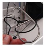
5. **Topping lift.** One of the awesome features of the Zim 420 is that the topping lift is one piece and when rigged properly your pole will not sky. The hook for the topping lift will need adjustment. Pass the line through the fairlead in front of the mast and through the fairlead to the left of the mast step. Once it passes through the bottom fairlead it should be attached to the shock cord. You may want to add a large stopper ball so the
