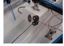
shackle to the boom bail as pictured below. The primary vang control line also needs to be connected. The primary is attached under the board cap. Take the loose end and place it through the lower vang block at the mast bail and up through the vang cleat and then into the fairlead.
