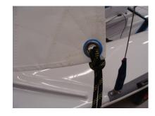
11. **Install the spinnaker**. Feed the spinnaker sheets through the spinnaker blocks. Keep the sheets forward of the traveler and outside the shrouds to meet with both ends forward of the forestay. Key point- Be certain the spinnaker sheets are outside of everything. The spinnaker has a head and 2 clews. Attach the head first by tying a bowline through the grommet. A bowline will then attach the spin sheets to both clews.
