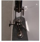
4. **Attach the trapeze rings.** Feed the shock cord retainer loop thru the small part of the ring and then take that same loop around the large ring at the base. Your boat may include a trap ring with a bullet block. If so, there is a hole just under the block for the shock cord to feed through.
