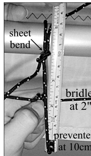
**Tie the sail on:** Lay the mast on the floor or grassy area. Next, slide the boom bling around the bottom of the mast and snap the boom jaw to the mast about 6" below the bling peg. Make sure the boom is right side up at this point as well and the vang cleat is directly under the boom. Now spread the sail out to fit inside the mast and boom with eyelets toward the spars.
