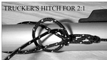
Next, secure the bridle to the aft bridle fitting with a trucker's hitch. Pull the trucker's hitch as tight as you possibly can. To finish it off, wrap the hitch with half hitches that draw the bridle even tighter. After the bridle is done, you will want to pull the bridle like an archery bow string and make sure it does not exceed the maximum of 10 cm from the boom (class rule). If it does, start over with the trucker's hitch and stretch it even tighter.
