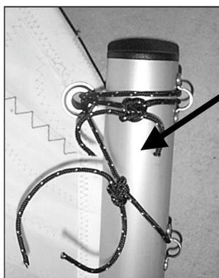
***Performance note:** Accordingly, the halyard preventer works in contravention to the sprit adjuster by positioning the sail band within the class legal bands on the mast. Tighten it to lower the sail. Loosen it to raise the sail. Keep in mind that after setting it, heavy vang and halyard adjustment can sometimes pull the sail past the mast bands and must be accounted for.*
