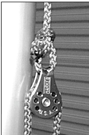
**Rig the Sprit Adjuster:** The sprit adjuster or halyard is a 2:1 purchase. This is a class rule. For the club rig, use the longer line to attach the Sprit to the purchase system. The loop from a bowline knot works as a cradle for the sprit tip. The shorter line is used to create the purchase. Tie one end to the bridge of the cleat and the other end is fed through the floating block and then through the cleat.
