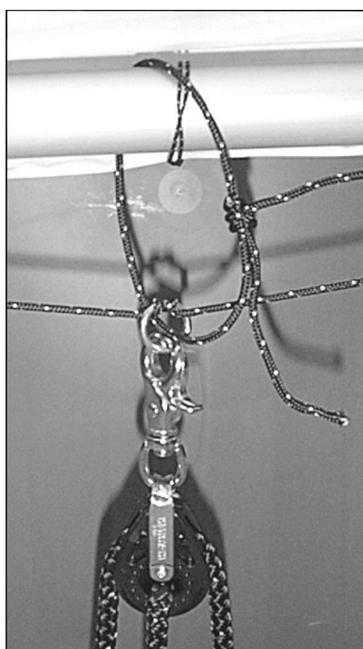
Once satisfied that the bridle is tensioned correctly, add the bridle preventer. The **bridle preventer** should restrict the bridle to pulling no more than 10 cm from the boom in the event it loosens. Tie the preventer with a sheet bend (a square knot would flip and loosen under tension).
