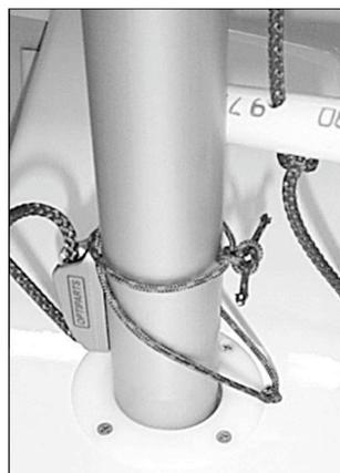
the rig must be transported any distance or if the wind is too strong, fold the boom up to the mast and carry it folded up.
