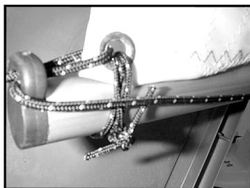
Finish up by tying the boom corner tie at the tack, followed by the loose intermediate boom ties (be sure to tie under the bridle or outhaul). Don't make the mistake of leaving off the clew corner tie and assume the outhaul will hold it down. This tie is just as important as all the others (see left pic).
