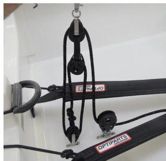
**Bowline:** Since the boat is for young kids, it is important to make sure the bowline is rigged and stored properly. The bowline dead ends at the mast step with a slip knot or tight bowline. If you use a bowline, make sure it's tight so it will not loop itself around the threaded adjustment rod. The boats are towed in a daisy chain configuration, so you also want to make sure there is a bowline on the bitter end of the line and it's coiled up and stuffed under the rail.
