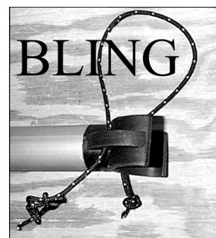
Next, add the **boom vang**. On the racing rigs, there might be a smaller line or wire that connects the vang adjustment line to the boom. On the club rig it is just a simple line and it can be secured to the boom with two half hitches or a doubled turn bowline. This will prevent it from riding over the vang peg toward the mast.
