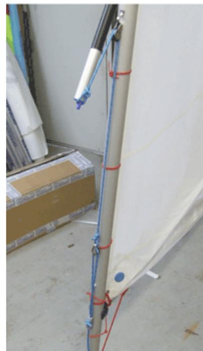
**Stepping the mast:** Most eight year olds are able to step the mast alone after a little practice. The trick is to keep the hands spaced wide apart on the mast. If
